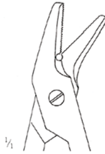
DI-05-131 12,5 cm / 5" Wire Cutting Scissors one toothed cutting edge
